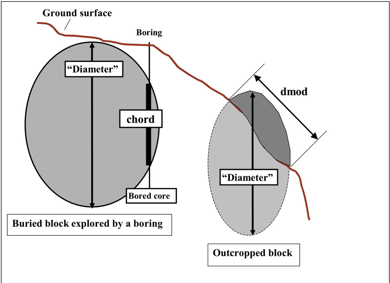
Figure B3. In two dimensions a block has apparent block size of  $d_{mod}$ , the maximum observed dimension. In one dimension, the block size is indicated by the chord length, or intercept between a boring and a block. Only rarely is  $d_{mod}$  or a chord length equivalent to the actual “diameter” or maximum dimension of a block, and hence block sizes are generally underestimated.
